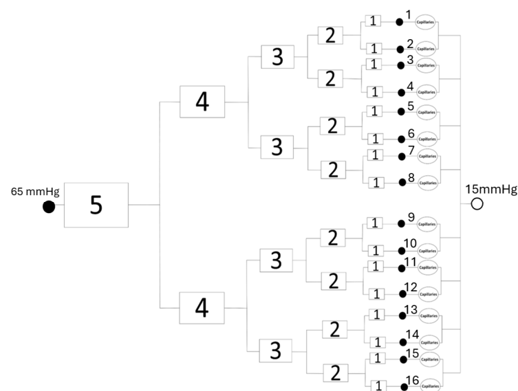
Figure 1. A simplified five-generation terminal arteriolar network with the lumped capillary bundle starts with 1 generation-5 arteriole and ends with 16 generation-1 arterioles and 16 capillary bundles. The blood pressure at the inlet of the network is 65 mmHg, and its value at the post-capillary venous side is 15 mmHg.
