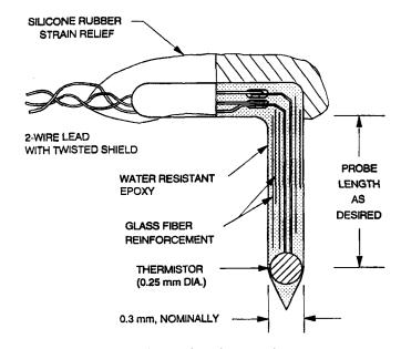
Figure 2. Sketch of a thermistor bead probe.
