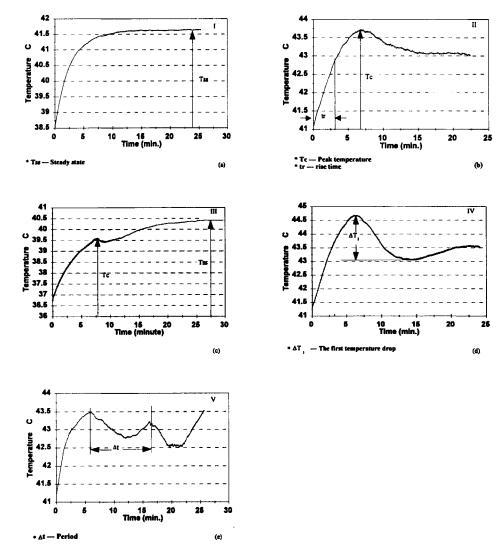
Figure 4. Five different types of tissue temperature response to the microwave heating observed in the canine prostate during transurethral hyperthermia treatment.
