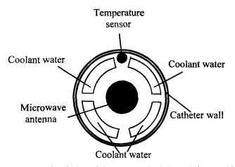
Figure 1. Cross-sectional view of the transurethral thermal therapy (T3) catheter (Urologix, Inc.)
