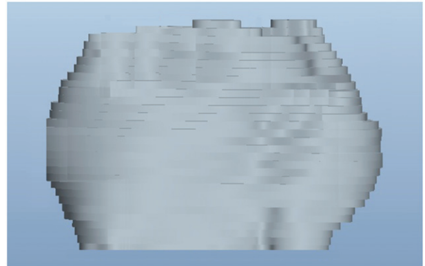
Figure 4. Prototype of the same tumour constructed in ProE ® from 30 microCT slices.
