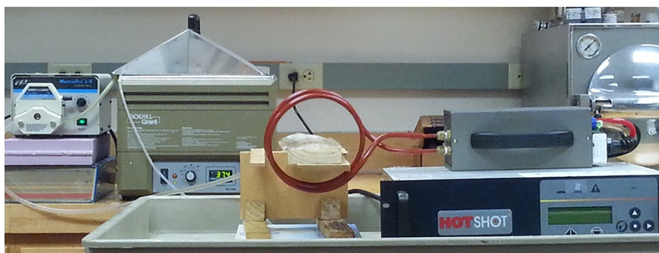
Fig. 1 Experimental setup of the study, including an RF generator, a two-turn coil to induce an alternating magnetic field, a stage for holding the mouse, a water circulating heating pad, a pump, and a water reservoir supplying 37 °C warm water
